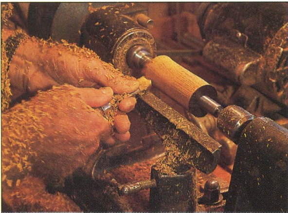
On the lathe the barrel is shaped mostly by eye. Dennis adds decorative cuts as well as a lanyard ring.
