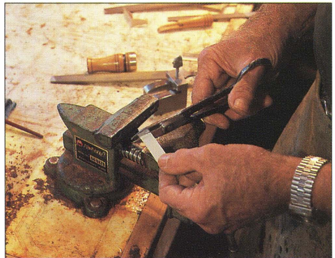
A strip of mylar is cut for the reed. Hand tuning each call, Dennis will chuck the insert if the right tone can't be found.
