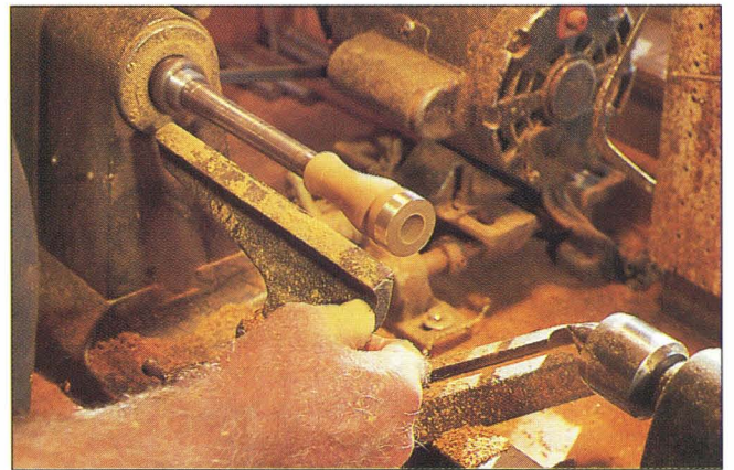
The signature brass ring is added, and the barrel is finely sanded and polished before Dennis starts the insert.
